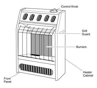
Figure 1 - Vent-Free Natural Gas Heater
